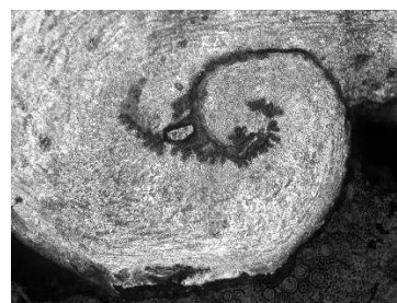
Obr.17 Detail nákrúžku z medi Fig.17 Detail of copper collar
