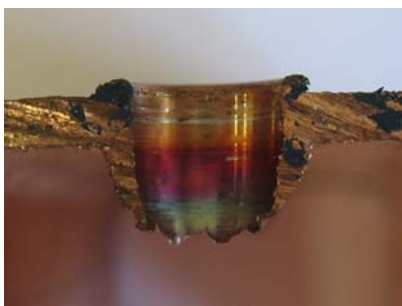
Obr.13 Medené puzdro , 2490 ot/min Fig. 13 Copper busher , 2490 sp/min
