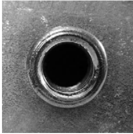
Obr.10 Závit- oceľ- 2490 ot/min Fig.10 Thread - steel – 2490 sp/min
