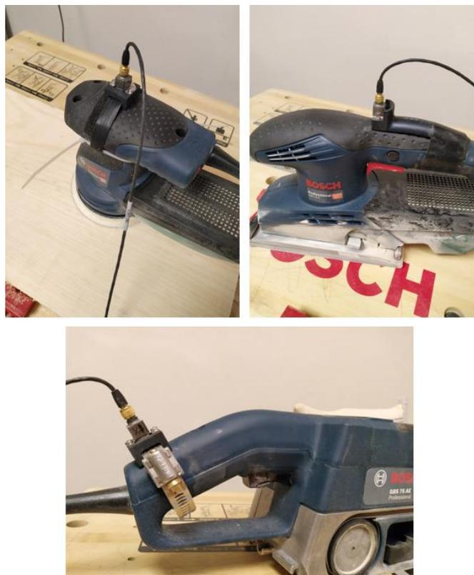
**Fig. 2 Location and mounting of transducer [5]**
