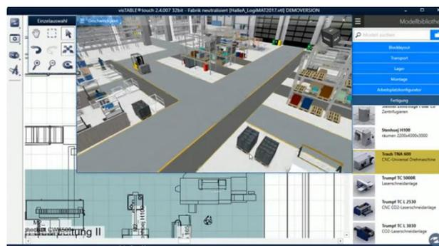
Fig. 2 3D visualization of a production hall in visTABLE®
