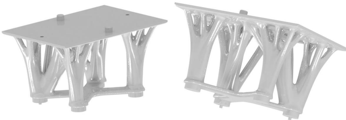
**Fig. 10. Table shape after topological optimization with Ansys Discovery software**
