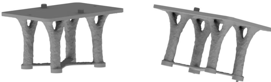
**Fig. 8. Table shape after topological optimization with Inventor Professional 2022**
