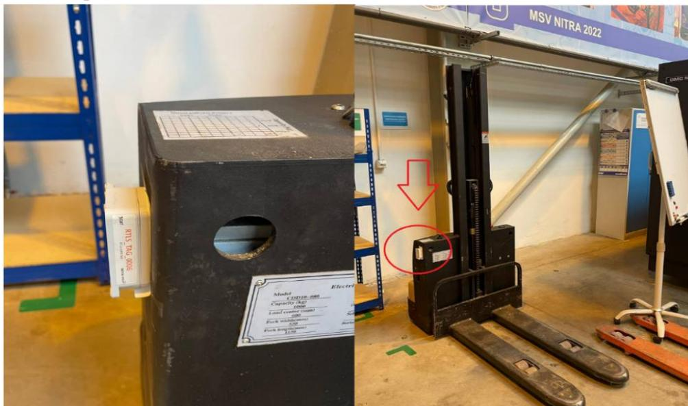
Fig. 3 RTLS UWB Wi-Fi Kit
