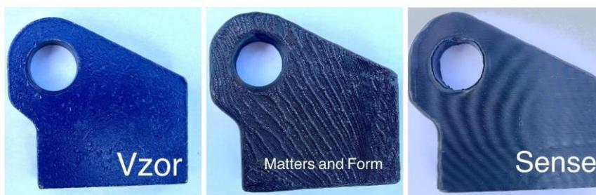
**Fig. 20** Comparison of the printed models with the pattern
