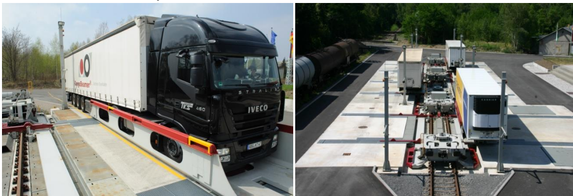
Fig. 3 Loading the semi-trailer and subsequent sliding onto the wagon in the terminal [1]
