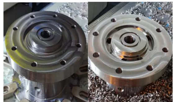
Fig. 6 Part after circular groove and pockets milling
