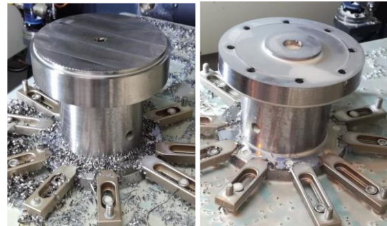
Fig. 5 Part clamping and face milling
