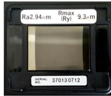
Fig. 2 Precision reference specimen
