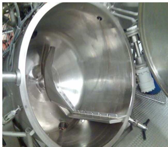
Figure 2 Opened mixer with a view on the NIR sensor and the mixing paddle
