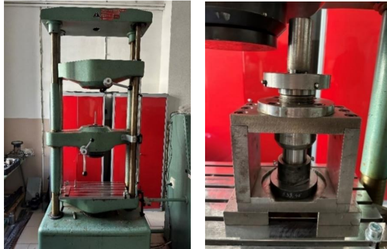
Figure 1. a) Hydraulic press ZD-40, b) experimental deep-drawing tool for cupping test
