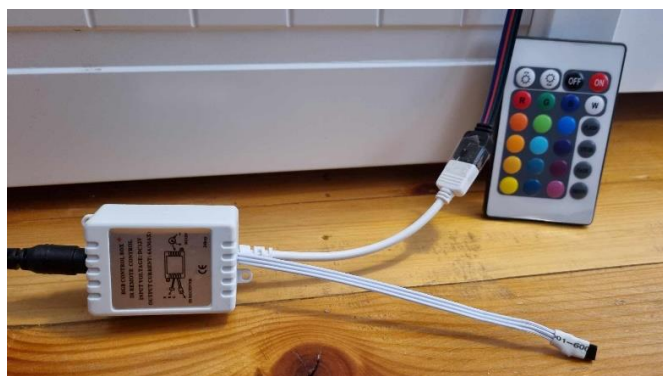
Figure 6. Controller for LED strip and power supply
