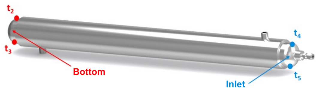
Figure 3. Position of individual temperature sensors on the tank.
