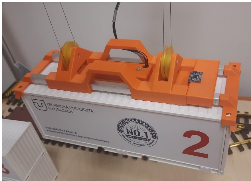
Figure 3. The accelerometer MPU6050 located on right side of spreader
