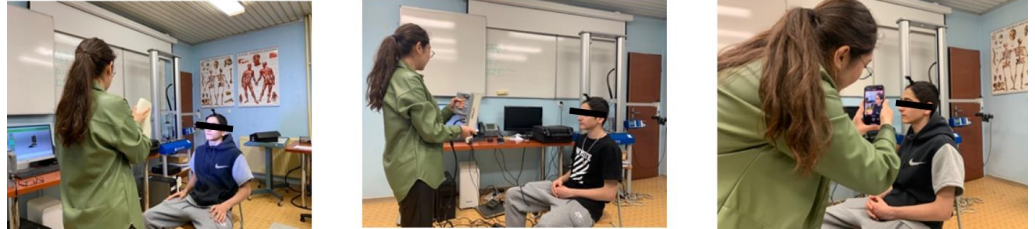
Figure 2. Face scanning of subjects (a) Artec Eva; (b) CR-Scan 01; (c) Scaniverse.
