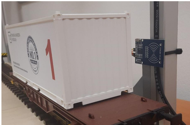
Figure 4. The RFID sensor reading of container tag
