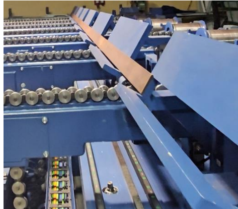
Figure 1. Photo of a fragment of a machine positioning a flat bar for measuring straightness.
