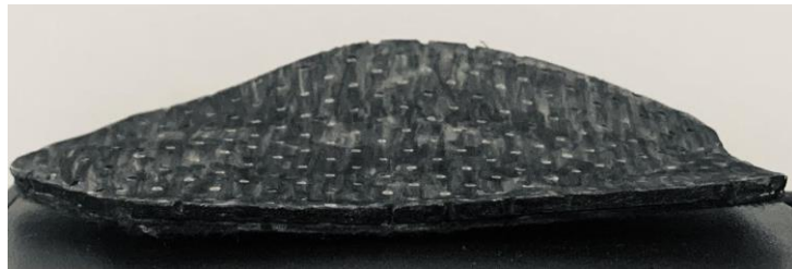
Figure 1: 3D foot orthosis (part of the orthopedic insole) in lateral projection, used orthosis sample.
