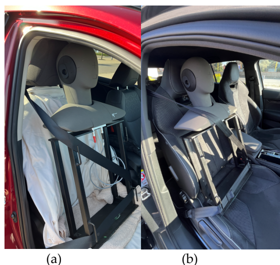
Figure 2. Placement of the psychoacoustic head in vehicles, (a) Toyota Rav4 hybrid, (b) Škoda Enyaq iv
