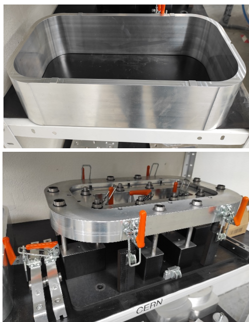
Figure 5 Utilization of the milling fixture in production
