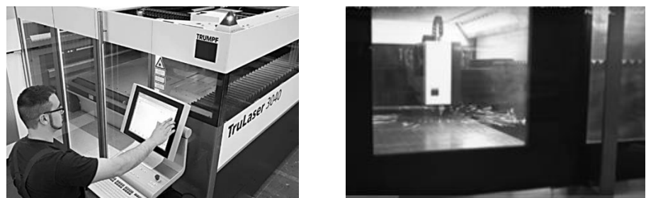
Figure 1. Laser cutting device during parameter input and material division [1,2].
