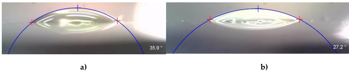
Figure 6. Outputs from contact angle measurements – a) Safety Lube 7815; b) Safety Lube 8801
