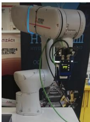
Fig. 2. Attaching 2D camera sensor to the robot Melfa Asista
