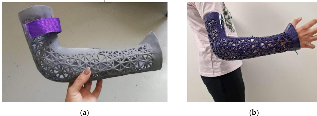
Figure 2. Final orthosis manufactured by MJF technology; (a) before postprocessing, (b) after postprocessing on the subject's arm.
