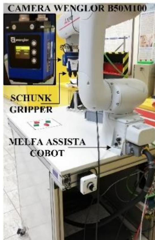
Fig. 4. The layout of the experimental collaborative workplace
