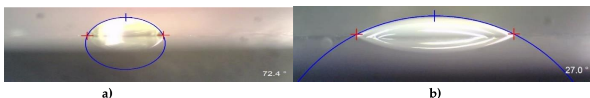
Figure 5. Outputs from contact angle measurements – a) Distilled water; b) Safety Lube 8801
