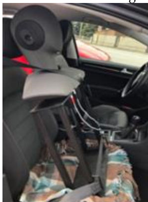
Figure 2 Placement of the psychoacoustic head in the vehicle
