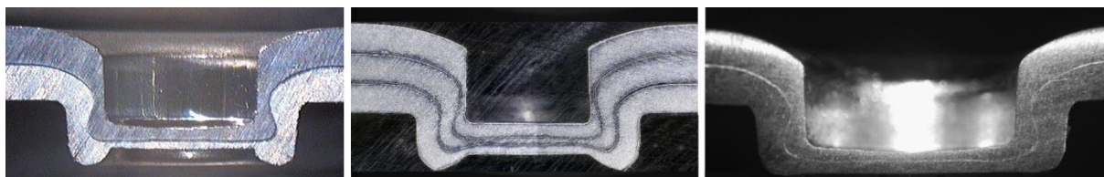
Fig. 2 Metallographic sections of various Clinching joints
