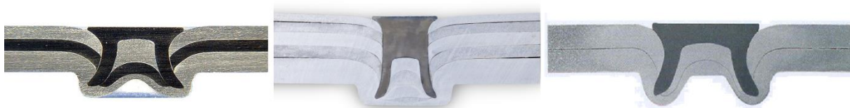
Fig. 4 Metallographic sections of various Self-piercing riveting joints
