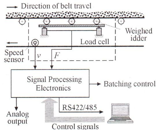
Figure 1 Principle view of a belt weigher
