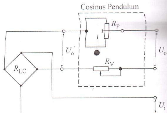
Figure 4 Variable belt inclination correction
