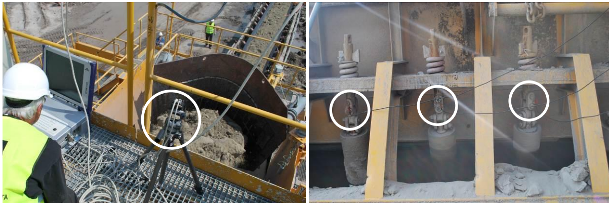
Figure 2 Vibration measurement – measurement device DEWE-5000 with high speed camera (left) and accelerometer placement on the impact rollers (right)
