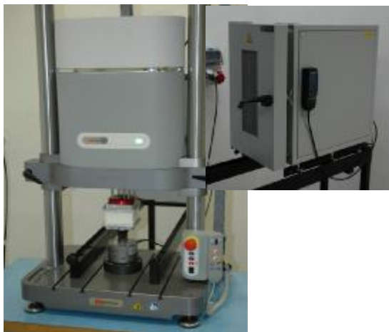
Fig. 3 Instron ElectroPuls 3000 and thermal chamber (TUL)
