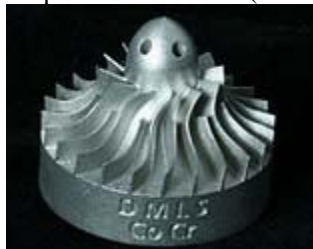
c.) Shot-peened with Metal & Ceramics ( R_a = 4 \mu\text{m} )
