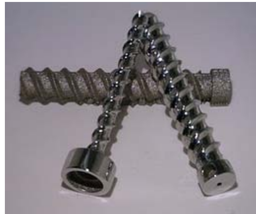
Fig. 6 Difference between raw material and finished part
