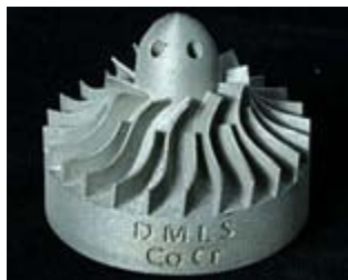
a.) As sintered ( R_a = 10 \mu\text{m} )
