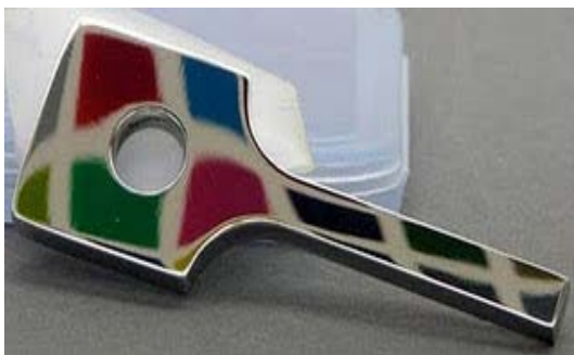
c) Cobalt Chrome MP1, optical polish with mirror finish
