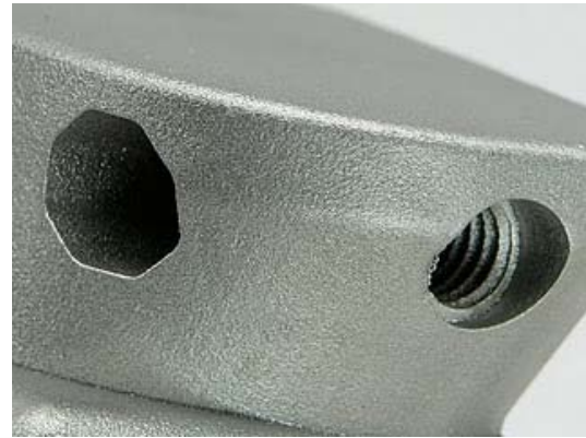
Fig. 4 Detail of shot peened finished surface, Stainless Steel PH1
