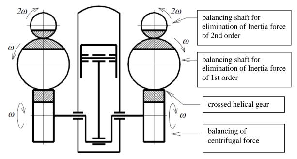
The Balancing goals: to reduce or eliminate the effects of inertial forces and their moments, which are manifested by oscillations, noise, fatigue, etc.
